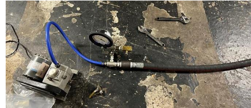
Fig. 6 - Bend Test of Vacuum Brake Hose.
